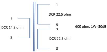
Figure 1. Wiring connections
