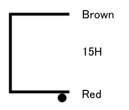
Inductance 15H Recommended DC current 180mA Max DC Current 240mA Minimum choke Input current 50mA DCR 146 ohm Max AC voltage 770V Dimension 80x71x120(H)mm Black hammered metal case, or Urushi finish Side screws are not in the dimension.
